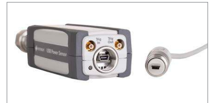
Figure 3. The external trigger input and output ports on the U2044XA.
